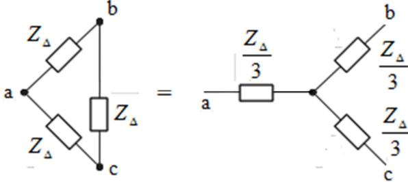
$$Z_{an} = \frac{Z_{ab} \cdot Z_{ca}}{Z_{ab} + Z_{bc} + Z_{ca}} = \frac{Z_{\Delta} \cdot Z_{\Delta}}{Z_{\Delta} + Z_{\Delta} + Z_{\Delta}} = \frac{Z_{\Delta}}{3}$$
